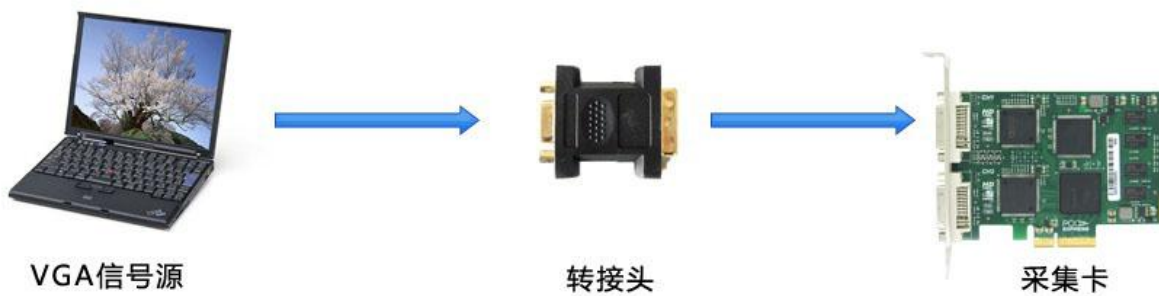
Figure 3, VGA signal connection sketch map
