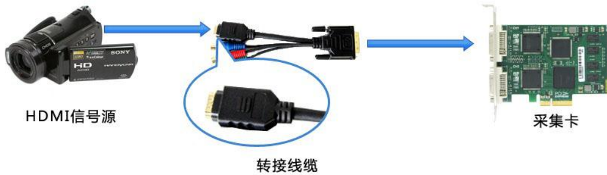
Figure 2, HDMI signal connection sketch map
