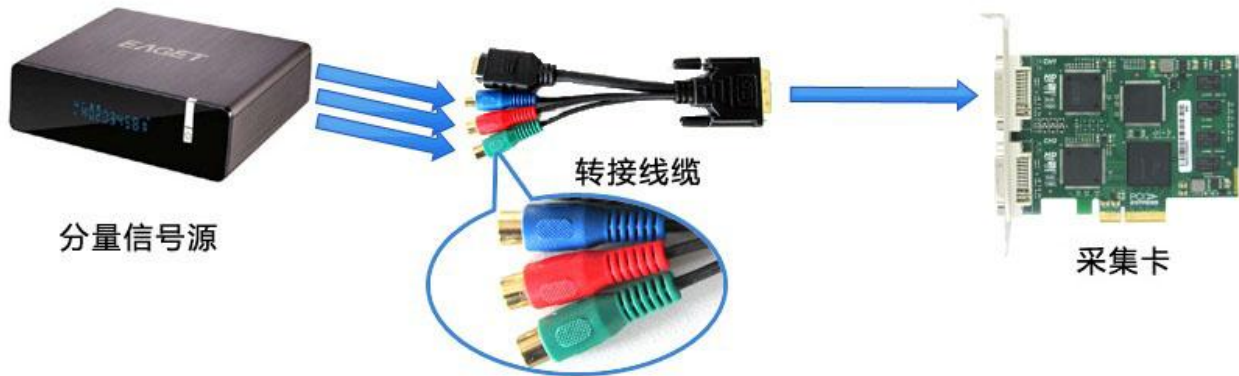
Figure 4, YPbPr signal connection sketch map
